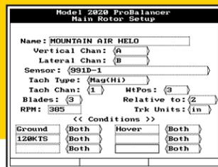
Configuration data such as the speed range, sensor requirements, and identification information can all be entered into a "Setup" and saved with a name such as "Mountain Air Helo." Later, if you need to analyze another Mountain Air Helo of the same configuration, you simply recall the saved Setup and begin the job. If a new configuration is needed, press the F1 function key and build a completely new setup. You can also make minor changes to a Setup, such as sensor type, with the edit function.
