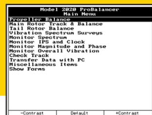
The Model 2020HR starts you off with an easy-to-understand menu. Simply pick what you want the analyzer balancer to do and press enter. Handy function keys just below the screen control common configuration changes so that you need not go into multi-layered menus to perform a minor task. The assignments of the function keys change as necessary with different screens to allow you to print, pause, continue, choose options, zoom, and do many other tasks.
