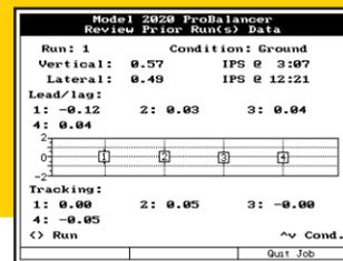
Each review screen contains all the information required to make adjustments to your job. The run number, condition, vibration amplitude/clock angle, and blade tracking information are recorded and readily available for viewing, printing, or storage with only a few keystrokes. Multiple jobs can be stored for various Setups for later review or reference. The data can also be transferred to a personal computer, enabling you to easily establish a database of the history of individual aircraft.
