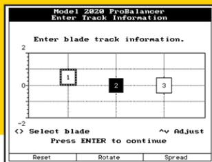
The track information screen, used in rotary wing applications, allows you to enter the blade track information manually, as shown in the example, from visual acquisition using a strobe, or it can be entered for you automatically by the optional Model 540-2 Optical Tracker System. This quick, "paperless" method of recording frees the user from data input. The track information is recorded and can be printed or recalled for later pitch link or tab adjustments.
