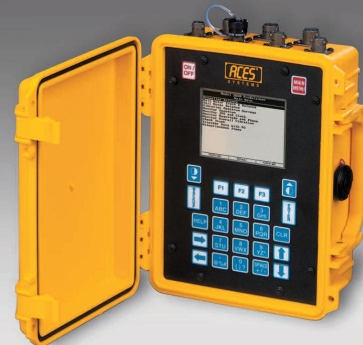
**The ACES Systems Model 2020HR ProBalancer Analyzer** combines the best features of previous ProBalancers with the spectrum analysis capabilities of our top-of-the-line ACES Analyzers. With its true, two-channel simultaneous inputs, the Model 2020HR makes performing twin engine propeller balancing a snap, as well as acquiring both vertical and lateral helicopter main rotor vibration measurements without switching channels.
