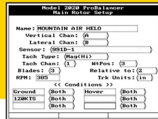
Configuration data such as the speed range, sensor requirements, and identification information can all be entered into a “Setup” and saved with a name such as “Mountain Air Helo.” Later, if you need to analyze another Mountain Air Helo of the same configuration, you simply recall the saved Setup and begin the job. If a new configuration is needed, press the F1 function key and build a completely new setup. You can also make minor changes to a Setup, such as sensor type, with the edit function.
