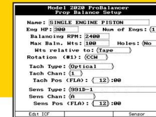
Should the information in the Setup change, for example the tachometer position, “Tach Pos (FLA),” then you can also edit the Setup to match that configuration. The ACES Systems Model 2020HR is so versatile it even remembers the frequency of use for all stored Setups and moves the Setups you use most often to the top of the selection list. You can also edit existing setups to make an entirely new setup, for example changing a two-bladed prop to a 3-bladed prop which requires new ICFs.
