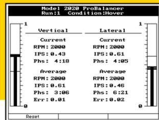
The full graphics capability of the Model 2020HR presents data in an easy-to-interpret format. As in the example screen, the IPS and clock functions appear in a "thermometer" format for easy viewing. Two channels are being acquired and displayed at the same time with independent IPS and Phase shown in both realtime and average. The analyzer even displays the percentage of error in the computation of the average. Pressing the F1 function key clears the running average and starts a new average.
