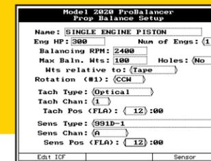
Should the information in the Setup change, for example the tachometer position, "Tach Pos (FLA)," then you can also edit the Setup to match that configuration. The ACES Systems Model 2020HR is so versatile it even remembers the frequency of use for all stored Setups and moves the Setups you use most often to the top of the selection list. You can also edit existing setups to make an entirely new setup, for example changing a two-bladed prop to a 3-bladed prop which requires new ICFs.
